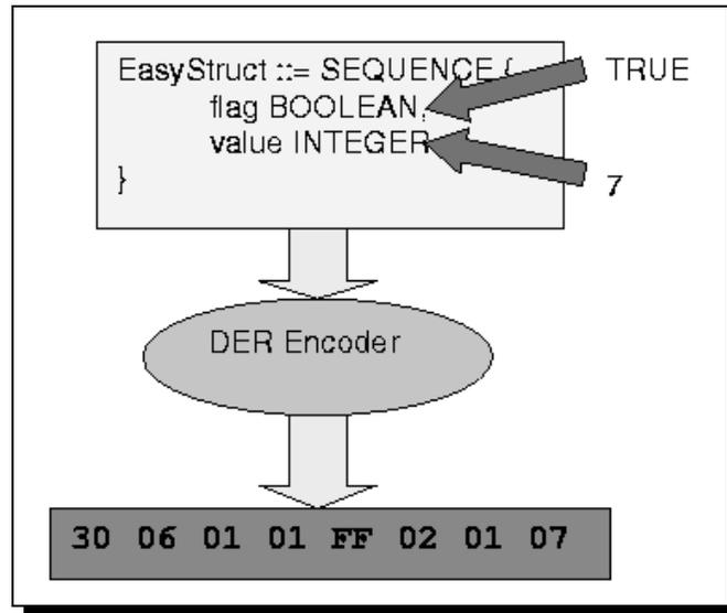
Figure 4: DER encoding of a simple data values of type *EasyStruct*.
